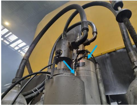
Figure 6 Plunger position measuring sensors a) Pressure measuring sensors b) located on the Diecasting machine
